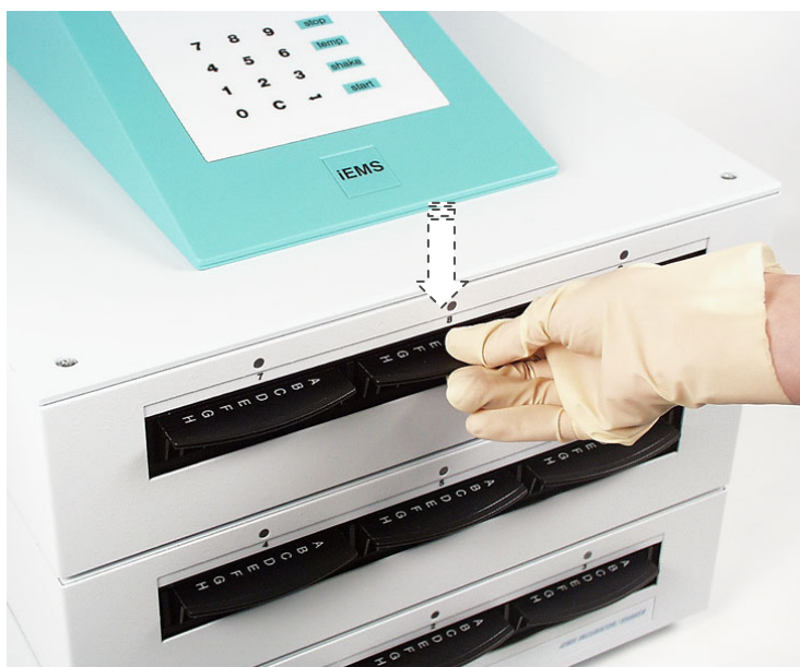
Fig. 6.4 Pushing down the microplate holder to latch it properly
