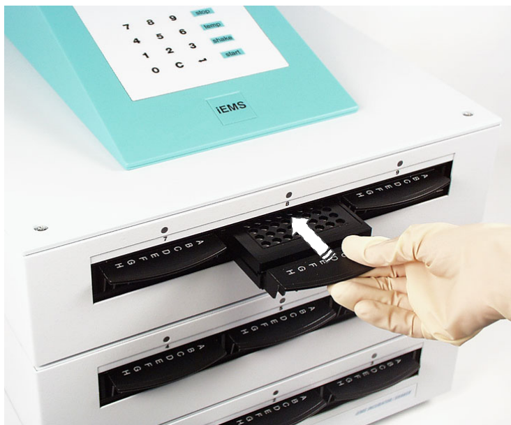
Fig. 6.3 Inserting the thermal microplate holder into a slot
